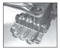
1. With a 22mm socket, remove the three discharge (43) and three inlet (41) manifold plugs. Check o-rings (42 and 44) for wear and replace as necessary.
