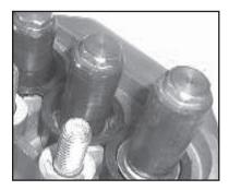
11.Inspect ceramic plunger (24A) tips for wear. If necessarv. replacement of the ceramic plungers may be accomplished by removing the plunger bolt assemblies (24B and 24C) with a 13mm wrench. Ceramic plungers should now slide off the stainless steel plunger base (22). Excessive resistance to plunger removal may be overcome by heating the stainless steel plunger base. This will melt any excess loc-tite beneath the ceramic plunger allowing easy removal.
