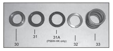
Inspect and clean the manifold (29) and pressure ring (32). Reinstall the pressure ring (30) with the groved side pointed towards the front. Insert v-sleeves (31/31A), support ring (32), and pressure spring (33) into the manifold.
