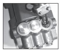
Using a small slide hammer remove valve seats (37) from manifold (29). Inspect valve plates (36) and valve seats (37) for wear. If excessive pitting is seen, replace the worn parts. Check valve seat o-ring (38) for wear and replace as necessary. Tighten manifold plugs (43) to 52 ft.-lbs. (70 Nm).
