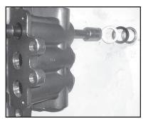
Turn the manifold (29) over. Using a 15mm socket, tap out the v-sleeves (31/31Afor P56W-HK), support rings (32), and pressure rings (30) through back of manifold.
