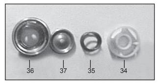
If pitted or worn, replace inlet valve seats (36), valve plates (37), springs (35) and spring retainers (34). Re-insert items 34-38 into valve adapter (39). Install valve assembly (34-40) into manifold (29). Reinstall manifold plugs (41) and torque plugs to 52 ft.-lbs. (70 Nm).
